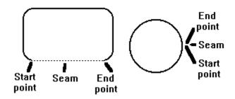
Each island is made up of a contour that has a start point and an end point. Between the start and end points is a seam which is usually very small (zero, in fact). When ROUGH chooses a path around the island, it will never touch the seam. Instead, the tool will run all the way around the other side of the island.
