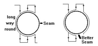
When the tool travels the long way around an island, all you need to do is move the seam. If you are using ROUND, then just alter the start angle.
