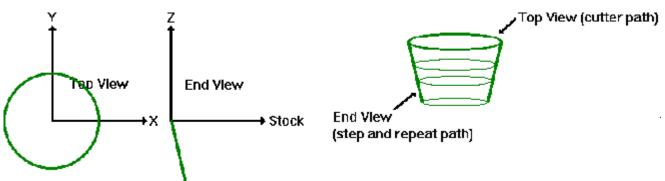
The End View starts at 0,0 and travels mostly down and slightly to the right. This tells +VIEW that as each step moves down in Z, more stock must be left on the walls. End Views almost always move down in Z. And unless you have a special undercutting cutter, End Views usually grow in STOCK. In other words, End Views almost always stay in the X plus and Y minus.
