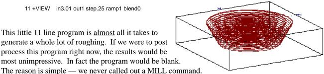
The post ignores everything before the first MILL command . Since the Views are for definition only, they will always occur before the first MILL. We use this area between a TOOL command and its first MILL command to hide things from the post processor. This area of source is called the "Dead Zone". So with a MILL added, the corrected source looks something like this:
