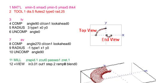
Note that we left ramping off in the +VIEW. Try turning ramping on and watch as your part gets sawed in half.
