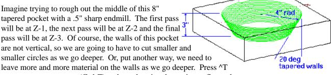
**RIGHT TRIANGLE** (Ctrl-T) and use the triangle routine to figure the taper amount:
