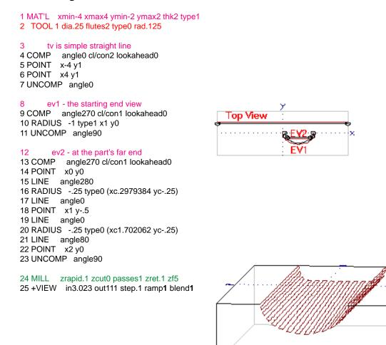
Ramp has extra power when used with a 3 View. It causes +VIEW to zigzag back and forth instead of lifting the tool and rapiding back to the start point.
