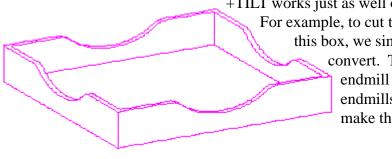
+TILT works just as well on geometry that is made up of radiuses. For example, to cut the XZ and YZ contours in the walls of this box, we simply program in XY and then let +TILT convert. To cut a shape like this, a very large ball endmill makes the going easier. Smaller endmills might require several passes in order to make the part's top flat.
