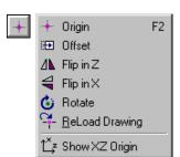
**OFFSET.** Offsets the origin of coordinates. You will be asked to "Enter the amount to offset the X-axis" and then "Enter the amount to offset the Z-axis."
